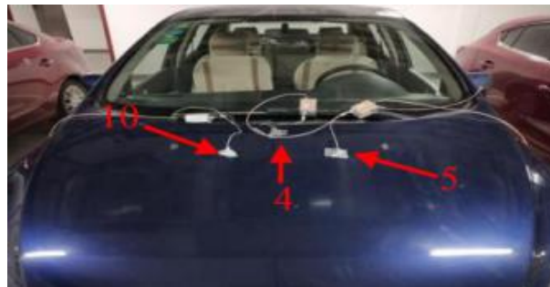
Fig. 6 The surface temperature measurement module on the hood
