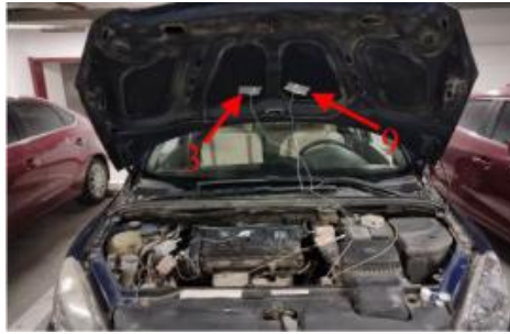
Fig. 8 The surface temperature module on the engine measurement module under the hood
