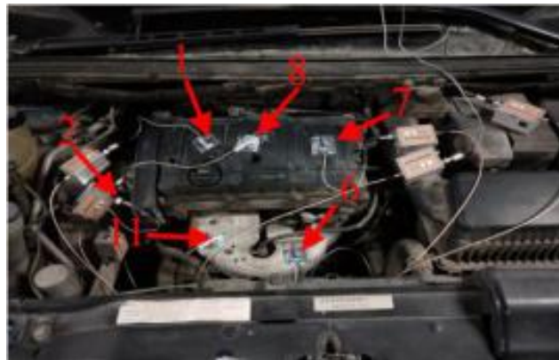
Fig. 7 The surface temperature measurement
